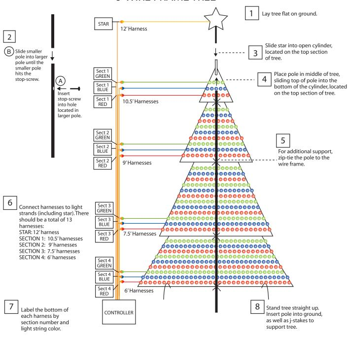
Plug each harness into the controller according to the suggestive diagrams to the right.
