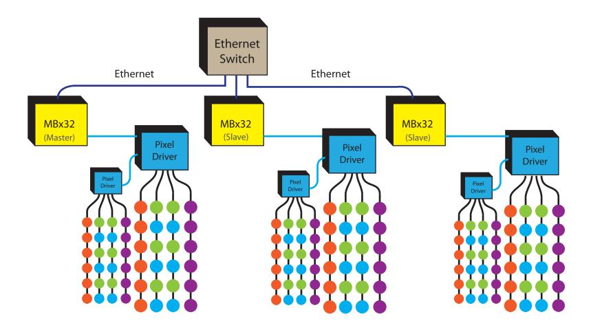
For our customers that require more than 2 Pixel Drivers, we use multiple MBx32 MonsterBrains networked together with an Ethernet switch. This allows us to connect as many Pixel Drivers together as we would like. We run these in what is called Master/Slave mode. A single MBx32 is chosen to be the master and that unit sends commands to all of the others. Very large networks can be achieved with ease.
