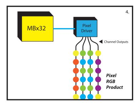
4. The newest technology that we offer at Animated Lighting is RGB Pixel control. Instead of the LC-16 light controller, RGB pixels require a controller called a Pixel Driver. The Pixel Driver controllers control our Pixel360, Pixy, Orb, Tube, Chip3 and Chip6 RGB products. Each bulb is individually controlled. Some of our Just Add Power RGB products include RGB Arches, RGB Stars and Snowflakes, 3D RGB Star and more. All of these products are controlled using the Pixel Driver.
