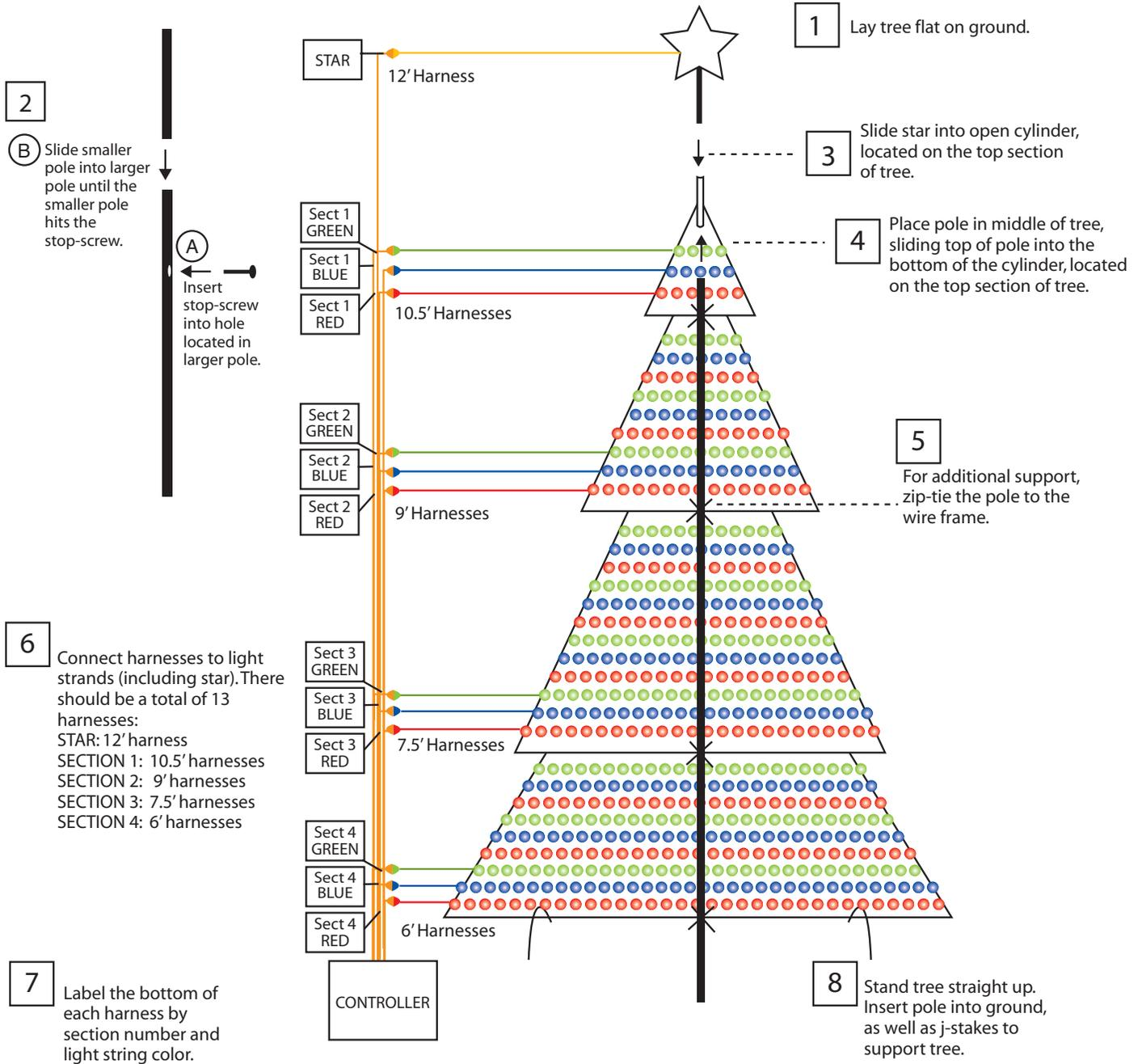
**9** Plug each harness into the controller according to the suggestive diagrams to the right.
