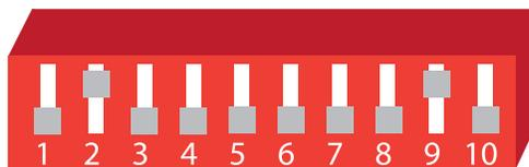
For newer pixel driver models, set the switches like this:
