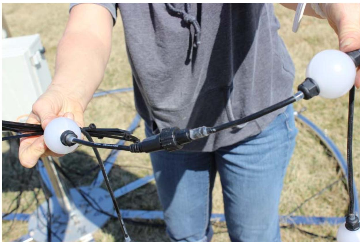
Then connect the male end of the two strings into the female connector labeled "1".
