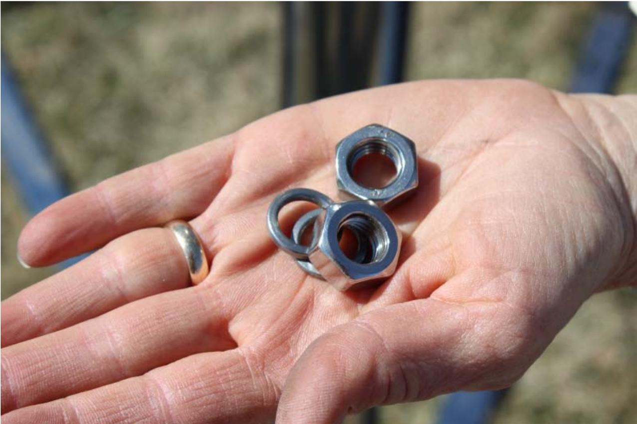
Tighten nuts. Note: two wrenches are required for this step.
