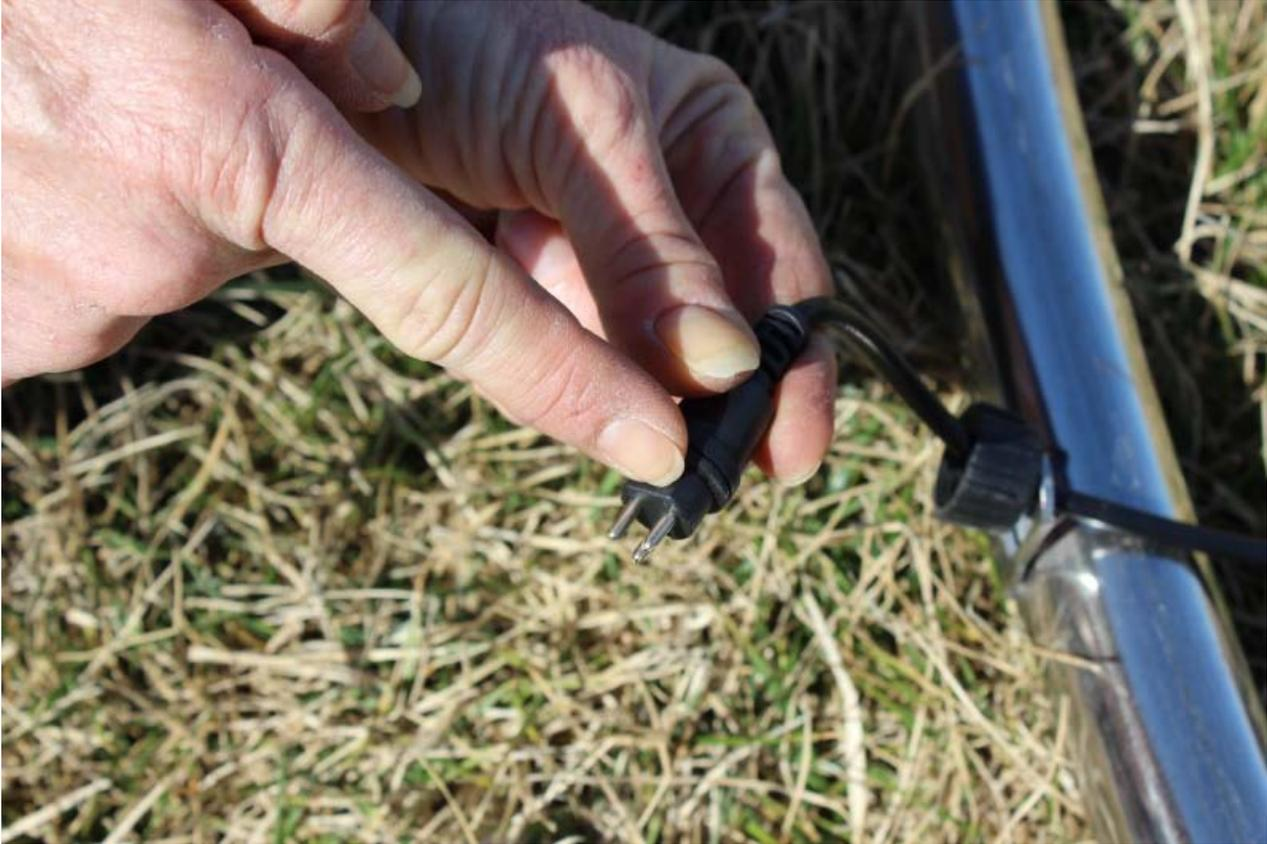
Connect the male POWER cable with the female at the "bottom" of the Tee and tighten the connection.
