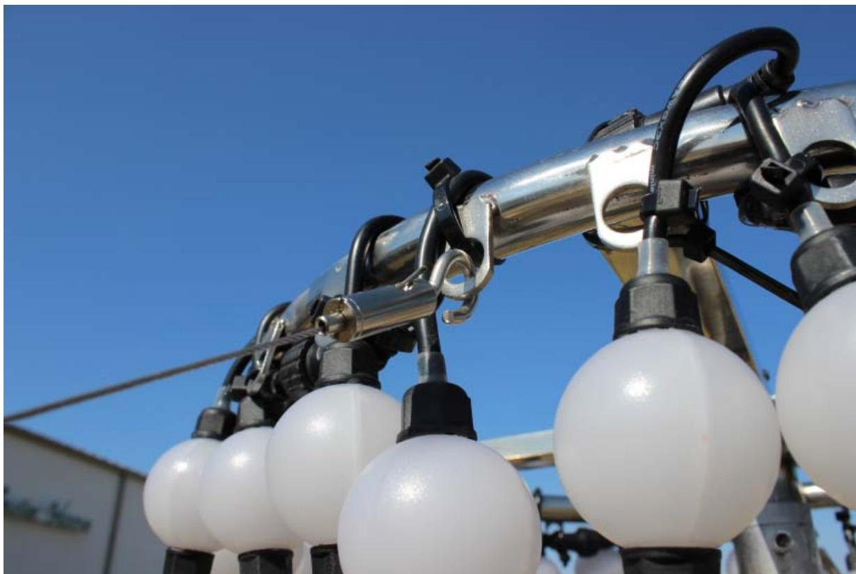
Make sure that none of your strings are going to snag in the process, then extend the telescopic pole by loosening the Allen bolt on the upper most section and extending it until the line is exposed.
