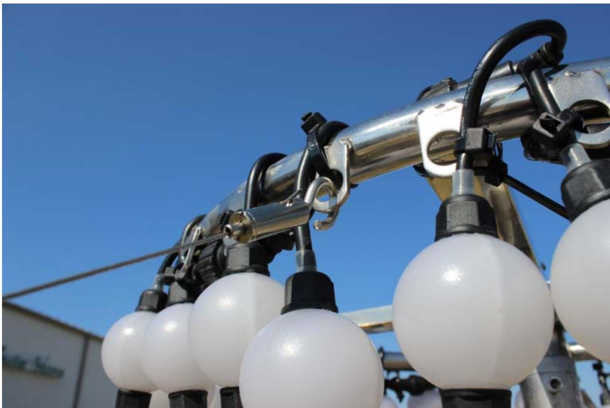
Make sure that all the cables are secured to the bottom of the frame with cable ties.
