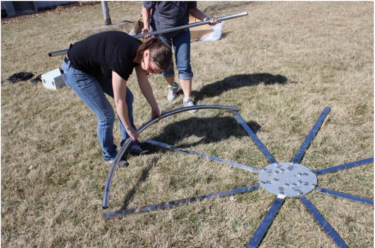
Match the labels and join the ring pieces with the spoke pieces using the Allen screws.
