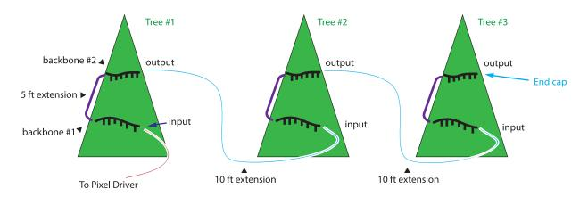
Step 8: Place the ORBs on the tree. As you put the ORBs in the tree, plug them into the backbone secured on the back. It is best practice to plug the ORBs into the backbone in the order that they are traveling up and down the tree.
