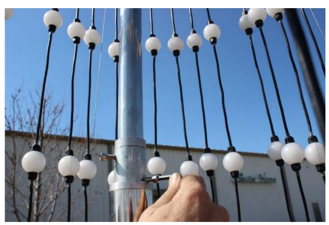
Once you see the line, tighten the top Allen bolt. Repeat this process until the telescopic pole is fully extended.
