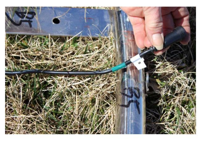
Notice the hooks near the edge of the lower ring. These hooks will connect our strings to the tree. Each cable coming from the controller will be assigned to a hook. The cable doesn't go in the hook, but needs to be placed near the hook. Not every hook will have a wire from the controller that goes with it. Only every OTHER hook will have a wire near it.
