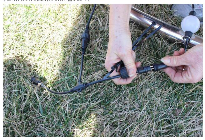
Repeat the process for the next 6 strings, but instead of connecting the first string to a single female cable (like Data 1), connect it to the remaining female connector on the Tee from the previous step.
