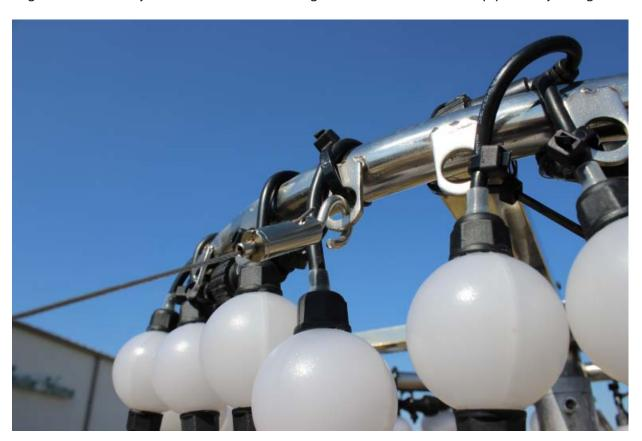
Make sure that all the cables are secured to the bottom of the frame with cable ties. Connect the controller to the MBx32 and test your light show!!
