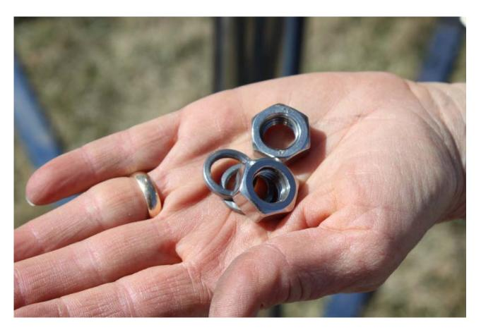
Tighten nuts. Note: two wrenches are required for this step.
