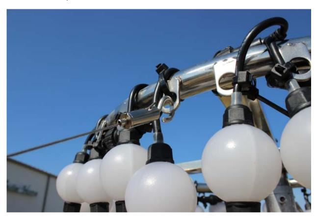
Make sure that none of your strings are going to snag in the process, then extend the telescopic pole by loosening the Allen bolt on the upper most section and extending it until the line is exposed. (This step will require at least 2 people)
