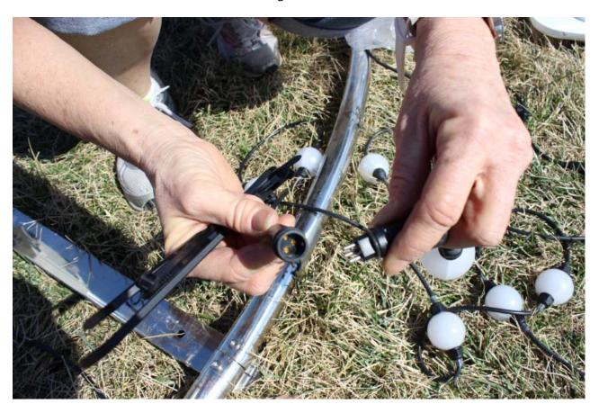
Take the center of the two strings (where you joined them together) and cable tie it to the nearest loop on the top ring. Each pair of strings should take up the space of two loops.
