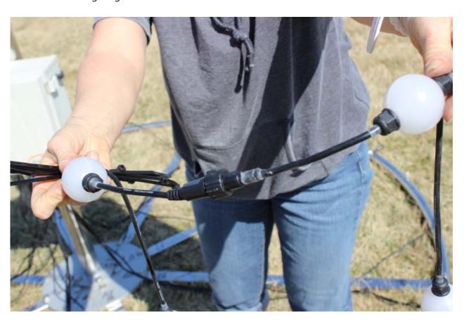
Then connect the male end of the two strings into the female connector labeled "1".
