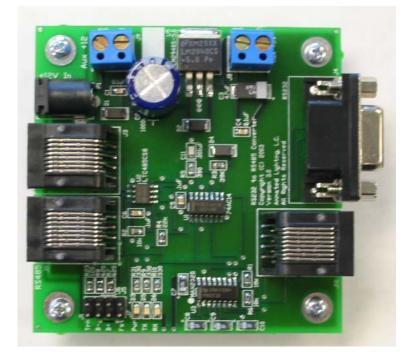
The RS485 Converter board is a bidirectional interface for converting RS232 signals to and from RS485 signals. It can be used in several configurations along with Animated Lighting's other controller boards.
