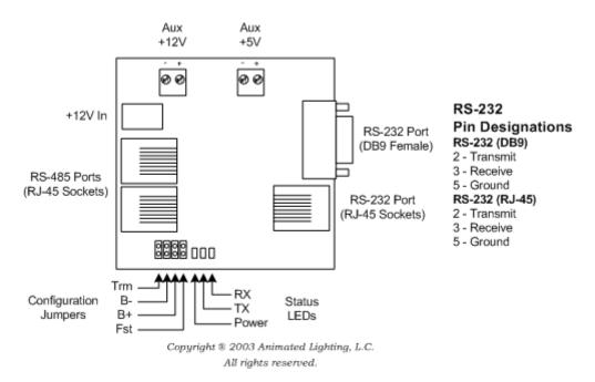
Power In - Power is typically supplied by a 12 volt DC wall power brick such as those sold by Animated Lighting. This 12 volts is also available on a terminal block to power low-current devices and is protected from reverse polarity connections. The 12VDC terminal block may also be used to power this board from another source (like a LC unit). See below for more information.
